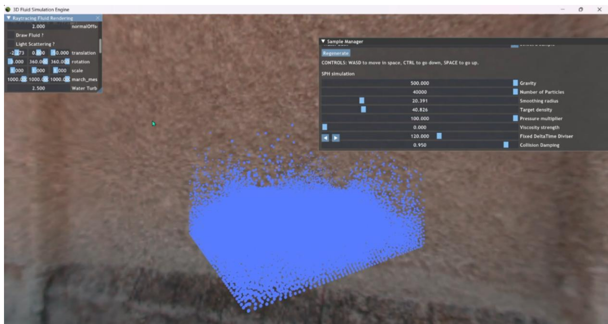
Figure 40 Screenshot of the fluid simulation with 40'000 particles after a significant Y-axis rotation, generating multiple splashes.
