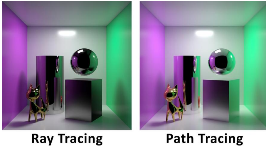
Figure 5 Comparison between ray tracing and path tracing. Image posted by Stampf on the Unreal Engine Forum (2022)
